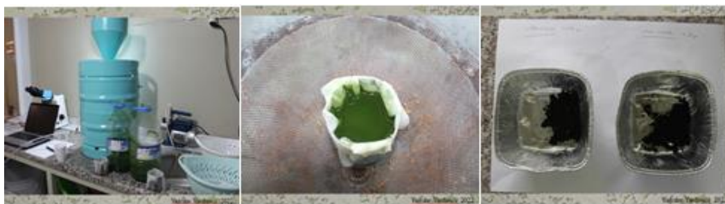
Figure 4. Filtration using a vacuum pump chamber or vacuumless with aluminum sulfate
